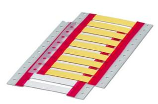
Marker for thermal transfer printer, unperforated, white, shrink sleeve for thermo transfer printer, unperforated, yellow, labeling field: 50 x 9 mm, can be used for 4.8 mm diameter, shrinkage ratio 3:1, 1 roll = 500 Marker at 50 mm
